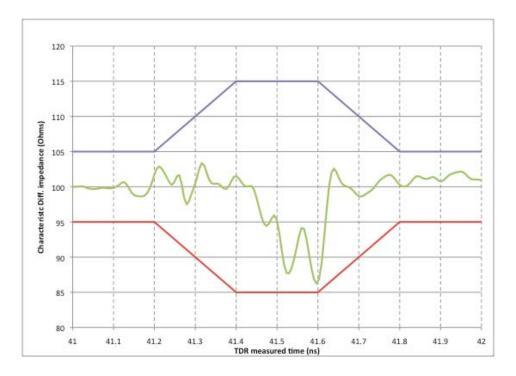
Figure 4-9: Mini DP Differential Impedance Profile Measurement Data Example
