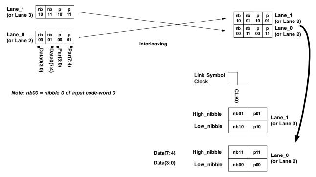
Figure 2-39: ECC Block Nibble-Interleaving for 2- and 4-Lane Main Links (Header)
