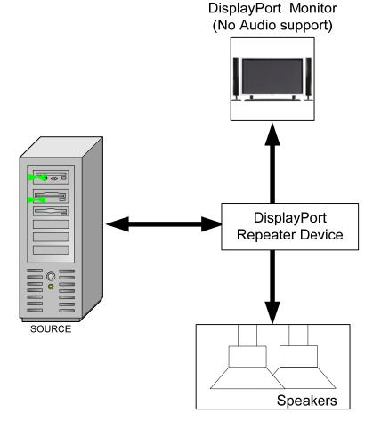
Figure 2-99: DisplayPort Monitor Connected Through a Repeater Device
