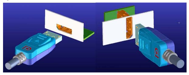
Figure 4-27: Recommended Orientation of External Connector
