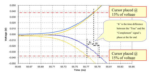
Figure 4-17: Intra-Pair Skew Measurement Method
