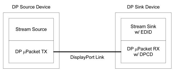
Figure 2-2: Single Link DisplayPort Link
