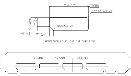
Figure 4-32: Panel Cut Out Reference Dimensions
