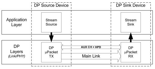
Figure 2-45: DisplayPort Data Transport Channels
