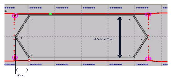
Figure 3-29: AUX CH EYE Mask for Manchester Transactions at Connector Pins of Transmitting Device
