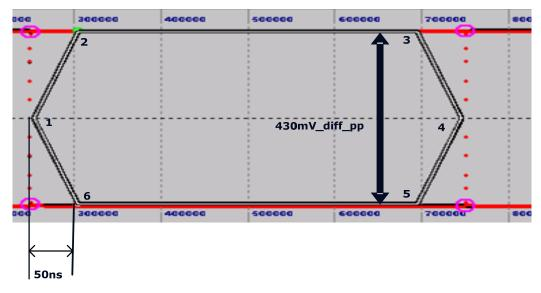
Figure 9-1: AUX CH EYE Mask at Transmitting IC Package Pins (Informative)
