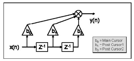
Figure 3-19: Feed-Forward Equalizer (FFE) Model
