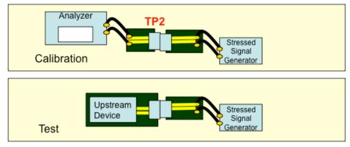
Figure 3-16: FAUX Back Channel Receiver Compliance Test Configuration
