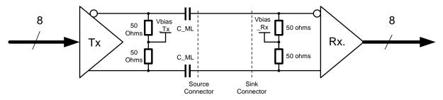
Figure 3-34: Main Link Differential Pair
