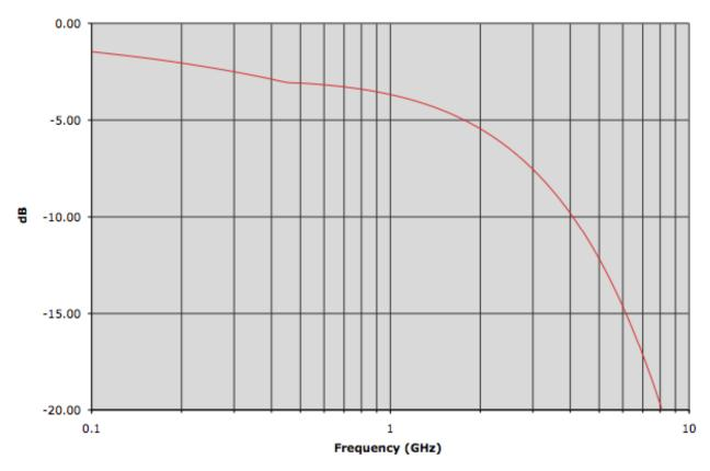
Figure 4-12: Mixed Mode Differential Insertion Loss for Extension Cable
