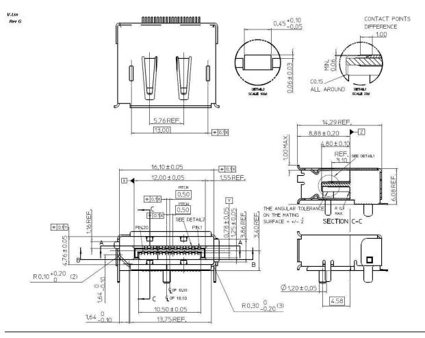
Figure 4-25: DisplayPort External Connector Drawings
