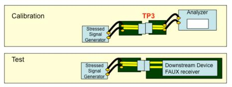
Figure 3-13: FAUX Forward Channel Receiver Compliance Test Configuration
