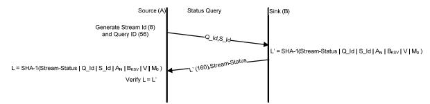
Figure 14-1: QUERY\_STREAM\_ENCRYPTION \_STATUS Message Transaction Execution when a Source Device is Directly Connected to an MST Sink Device
