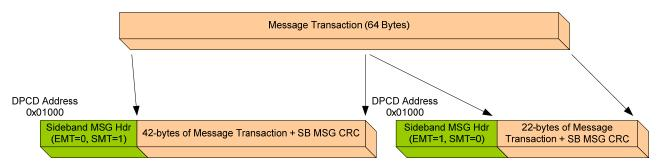
Figure 2-94: Mapping Message Transaction to Multiple Sideband MSGs (SB MSG CRC is the Sideband\_MSG\_Data\_CRC field.)
