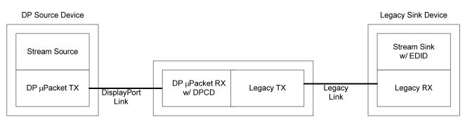
Figure 2-4: DisplayPort Source Device to Legacy Sink via DisplayPort-to-Legacy Converter
