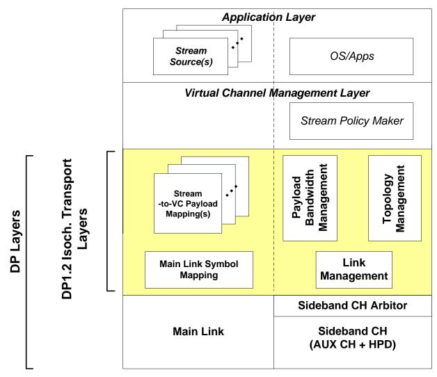
Figure 2-51: MST Isochronous Transport Service Layers
