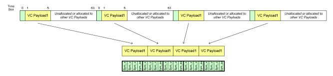
Figure 2-70: Repetition of 4-symbol Sequence Unit Example for 1-lane Main Link
