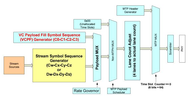
Figure 2-68: VC Payload Symbol Generator of a DP Source Device
