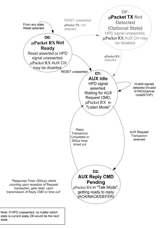
Figure 2-44: AUX CH uPacket RX State Diagram
