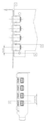
Figure 4-46: Reference Design for Four Mini DP Connectors on a Reduced Height PCI Card - 2
