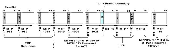
Figure 2-86: MSTM ECF and LVP Signaling at Link Frame Boundary
