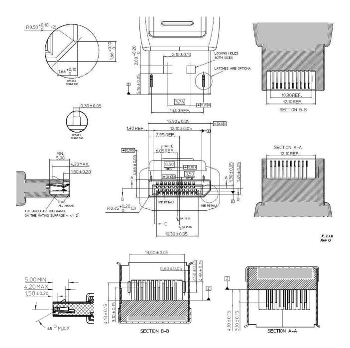
Figure 4-26: DisplayPort External Cable-Connector Assembly Drawings
