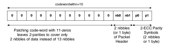
Figure 2-42: Makeup of 15 Nibble Code-Word for Packet Header
