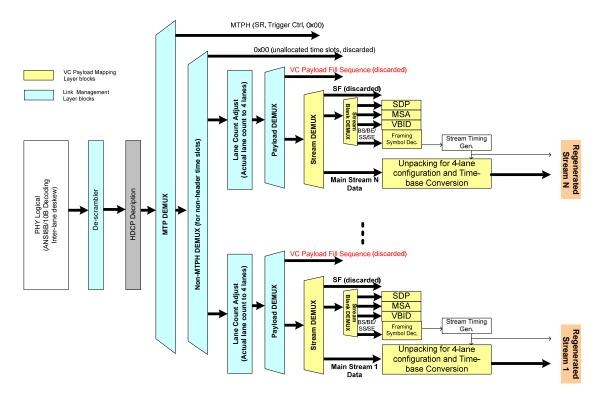
Figure 2-62: Logical Block Diagram of MST DP Sink Device
