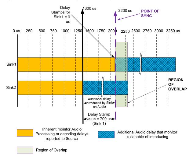
Figure 2-103: Delay Compensation for Audio-to-Audio Sync
