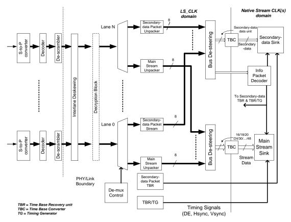
Figure 2-9: High Level Block Diagram of DP uPacket RX Main Link Data Path
