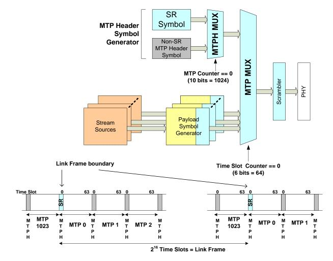
Figure 2-66: Link Timing Generation in MST Mode
