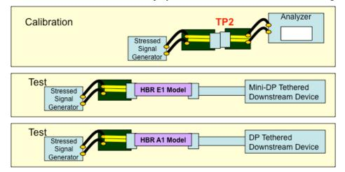
Figure 3-8: HBR Tethered Downstream Device Compliance Test Configuration
