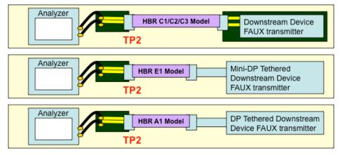
Figure 3-15: FAUX Back Channel Transmitter Compliance Test Configuration
