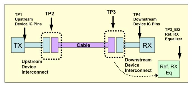
Figure 3-2: Compliance Measurement Points of the Channel
