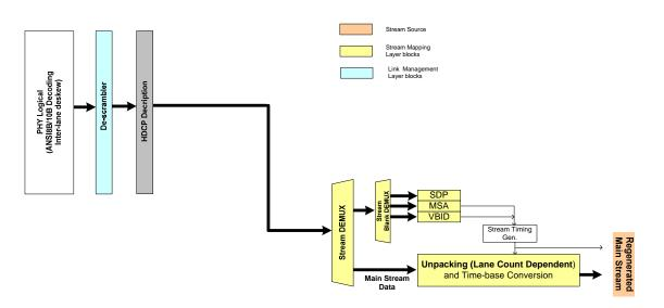
Figure 2-65: Logical Block Diagram of SST DP Sink Device
