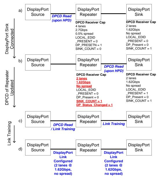
Figure 5-3: Action Flow upon Addition of Sink Device
