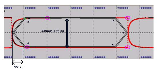
Figure 9-2: AUX CH EYE Mask at Receiving IC Package Pins (Informative)
