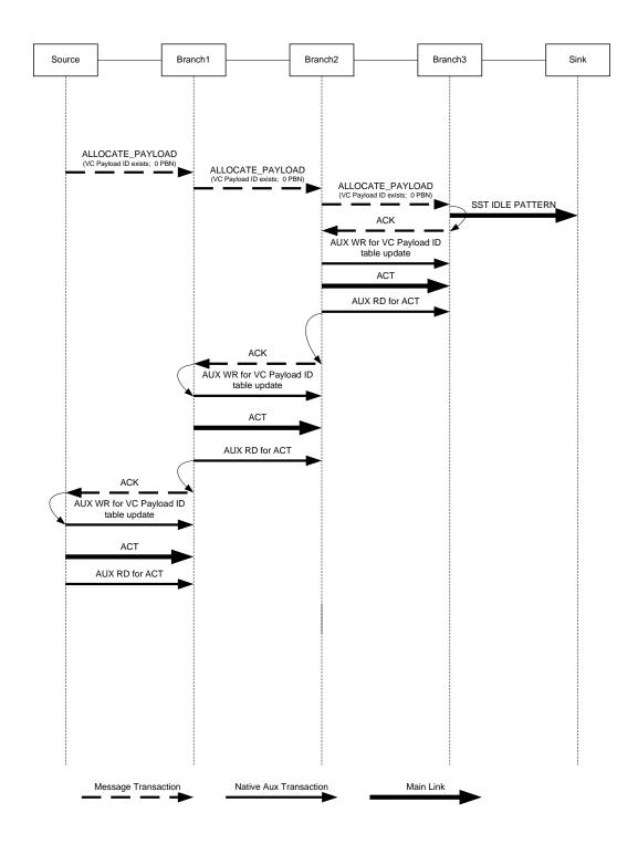
Figure 2-81: Timing Sequence for Deleting a Payload
