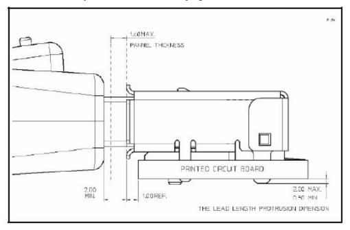
Figure 4-29: Fully-Mated Condition for DisplayPort External Connectors
