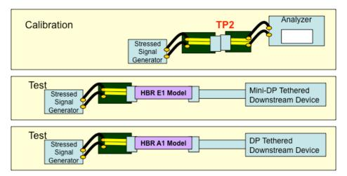
Figure 3-11: RBR Tethered Downstream Device Compliance Test Configuration
