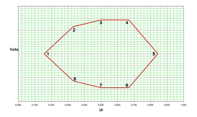
Figure 3-38: EYE Mask at Upstream Device Connector Pins
