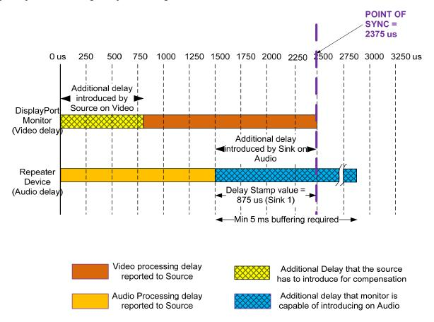
Figure 2-100: Delay Compensation for Audio-to-Video Synchronization
