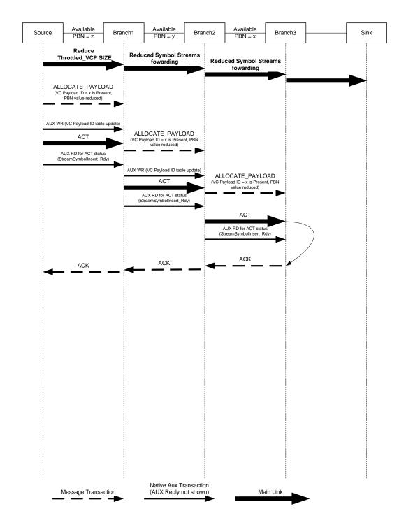
Figure 2-84: Timing Sequence for Reducing the VC Payload Allocation
