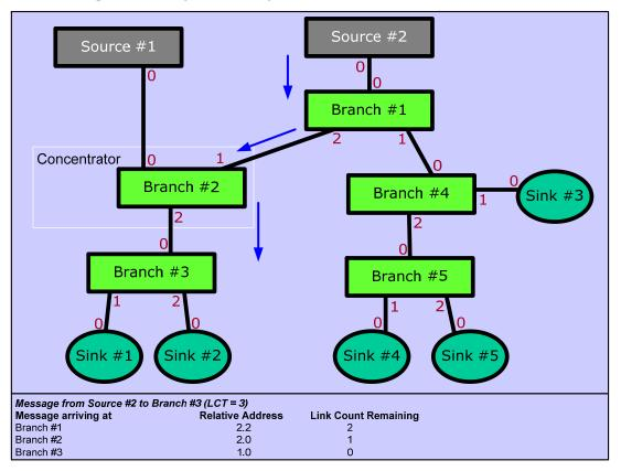
Figure 2-95: RAD Update Along the Path Using Example Topology
