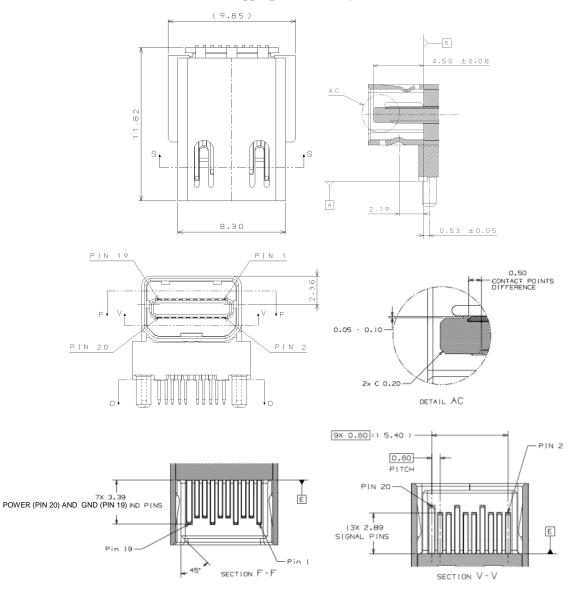
Figure 4-41: Mini DisplayPort Connector Dimensions - 1
