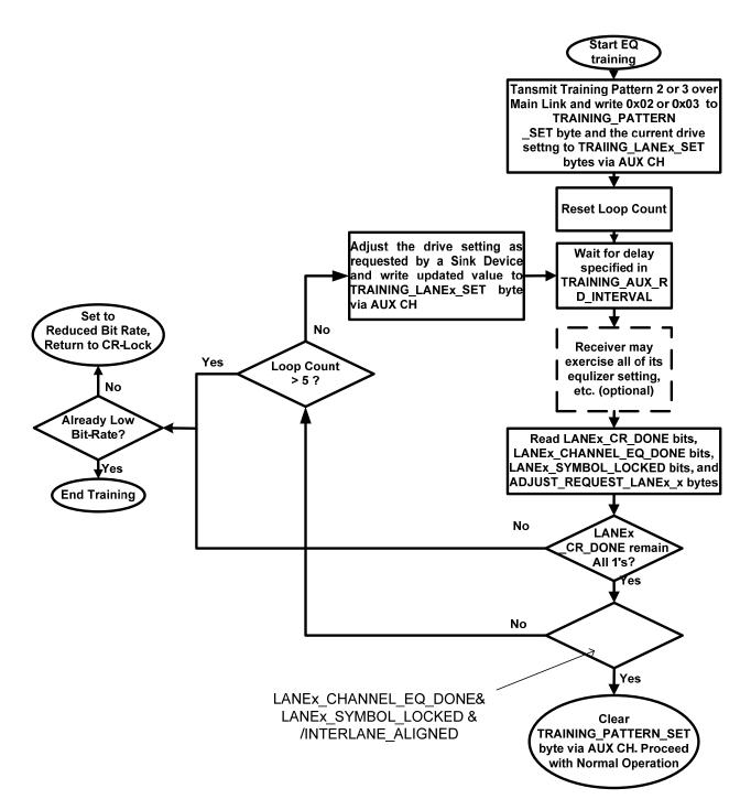
Figure 3-33: Channel Equalization Sequence of Link Training
