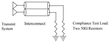
Figure 3-3: Compliance Test Load
