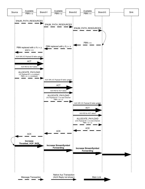
Figure 2-85: Timing Sequence for Increasing the VC Payload Allocation
