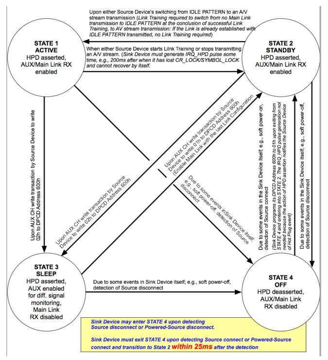
Figure 5-2: Sink Power State Machine
