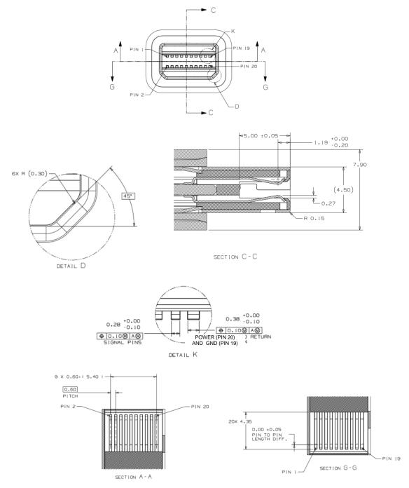
Figure 4-39: Mini DisplayPort Cable-Connector Dimensions – 1
