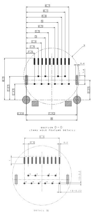
Figure 4-44: Recommended Mini DisplayPort Connector PCB Contacts and Mounting
