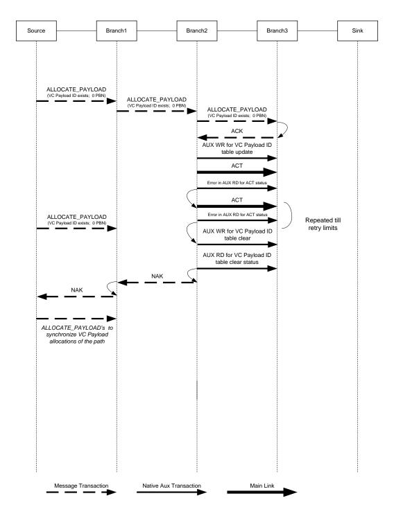
Figure 2-83: Timing Sequence for Deleting a Payload with Locally Unrecoverable Error
