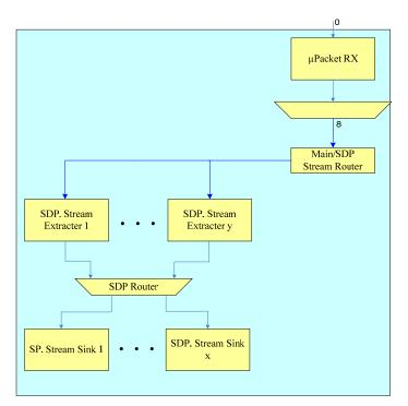
Figure 2-56: MST Audio-only Sink Device with SDP Sinks
