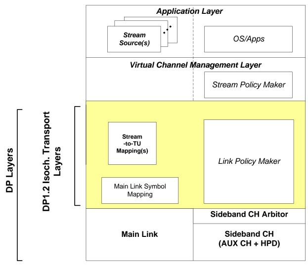
Figure 2-50: SST Isochronous Transport Service Layers
