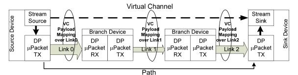
Figure 2-47: Illustration of Link, Path, Virtual Channel
