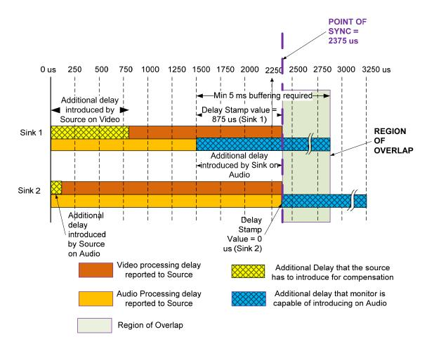
Figure 2-102: Delay Compensation for Audio-to-Video Sync in a Multi-Monitor Configuration
