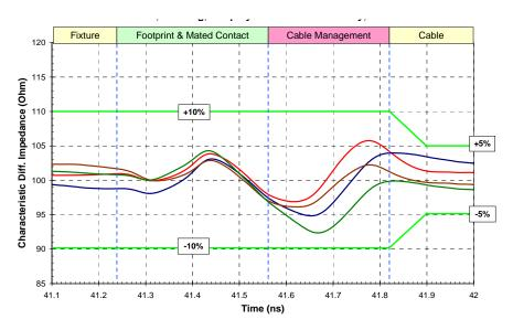
Figure 4-8: Differential Impedance Profile Measurement Data Example
