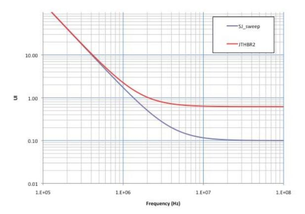
Figure 3-35: HBR2 Receiver Jitter Output/Input Tolerance Mask
