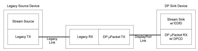
Figure 2-5: Legacy Source Device to DisplayPort Sink Device via a Legacy-to-DisplayPort Converter
