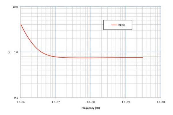
Figure 3-37: Reduced Bit Rate Jitter Output/Input Tolerance Mask
