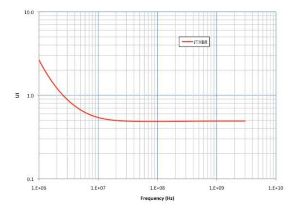
Figure 3-36: High Bit Rate Jitter Output/Input Tolerance Mask
