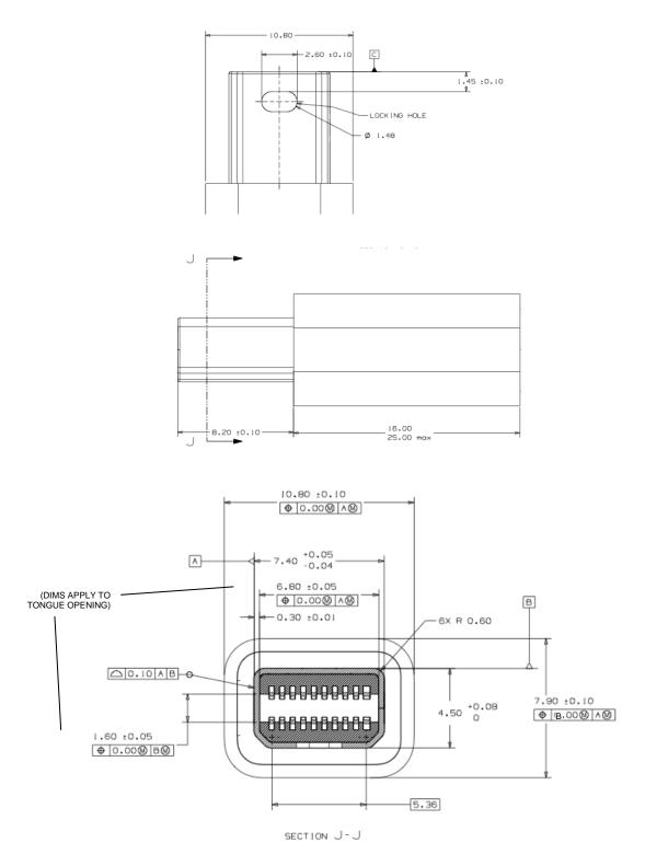
Figure 4-40: Mini DisplayPort Cable-Connector Dimensions – 2
