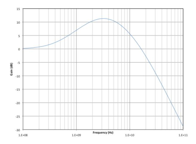
Figure 3-41: Reference HBR2 Receiver Equalizer Transfer Function
