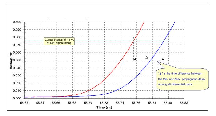
Figure 4-18: Inter-Pair Skew Measurement Method
