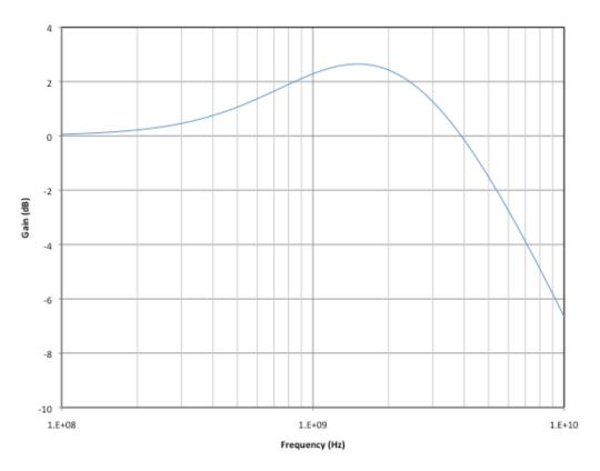
Figure 3-40: Reference HBR Receiver Equalizer Transfer Function
