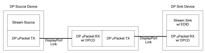
Figure 2-3: DisplayPort Source Device to DisplayPort Sink Device via a Repeater
