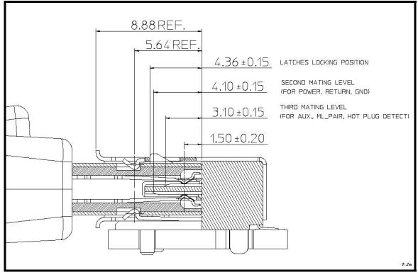
Figure 4-24: Connector Mating Levels
