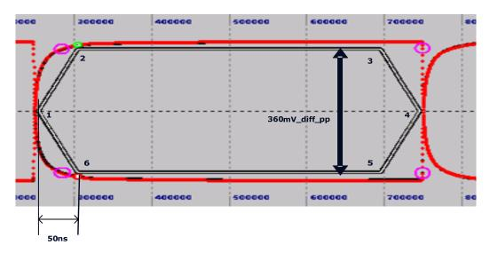
Figure 3-30: AUX CH EYE Mask for Manchester Transactions at Connector Pins of Receiving Device
