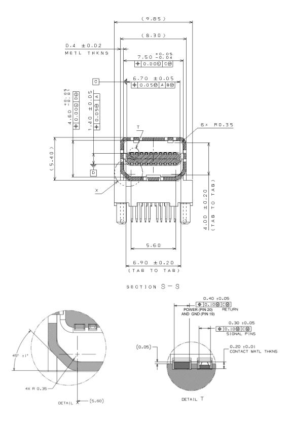
Figure 4-42: Mini DisplayPort Connector Dimensions – 2
