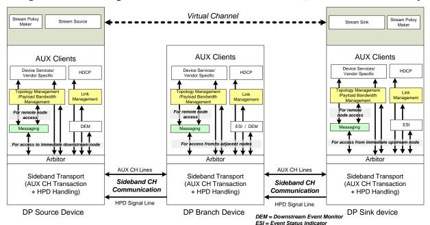
Figure 2-52: Sideband CH Communication Layers
