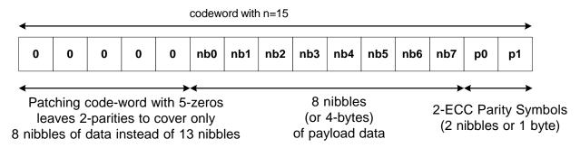
Figure 2-41: Makeup of 15 Nibble Code-Word for Packet Payload
