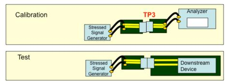
Figure 3-10: RBR Downstream Device Compliance Test Configuration
