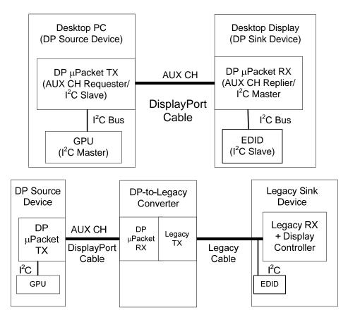
Figure 2-88: Examples of AUX CH Bridging Two I<sup>2</sup>C Buses
