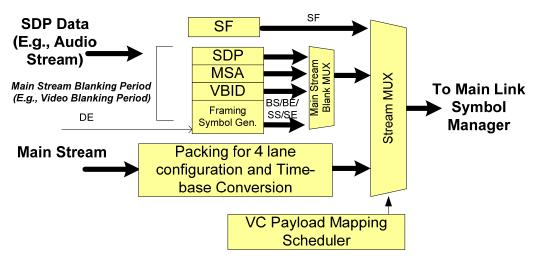
Figure 2-72: DP Source Device VC Payload Mapping Logical Block Diagram
