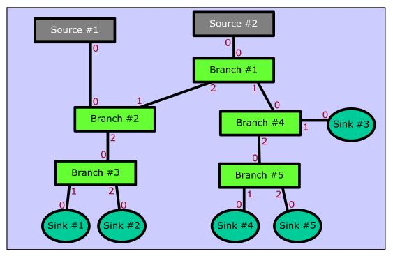
Figure 2-57: Example MST (Multi-stream Transport) Topology
