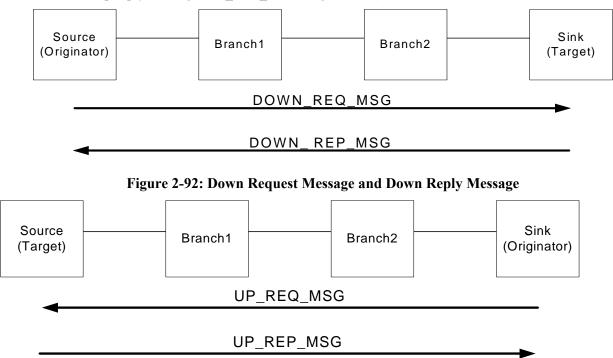
Figure 2-93: Up Request Message and Up Reply Message
