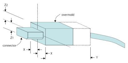
X: max 10mm from connector centerline
