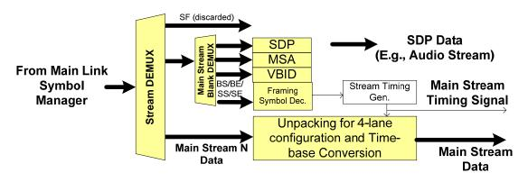
Figure 2-73: DP Sink Device VC Payload Mapping Logical Block Diagram
