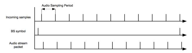
Figure 6-1: Audio Stream Packets Transfer with No Video or During Video Vertical Blanking
