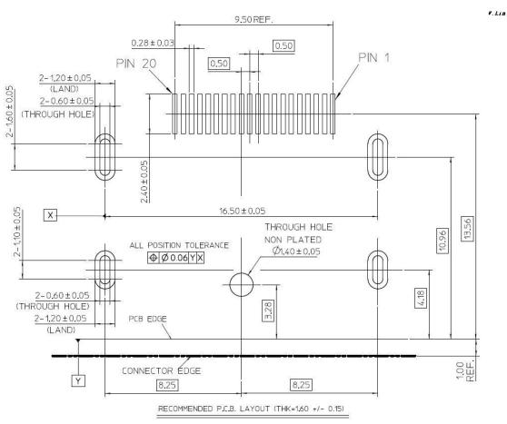
Figure 4-30: Recommended PCB Layout for DisplayPort External Connector
