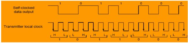
Figure 3-23: Self-clocking with Manchester-II Coding
