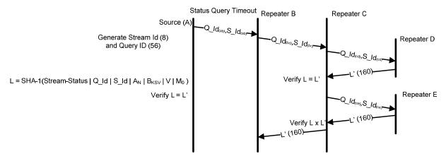
Figure 14-3: QUERY\_STREAM\_ENCRYPTION \_STATUS Message Transaction Forwarding and Execution when L-to-L' Verification Error Present
