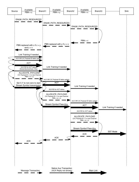
Figure 2-79: Example Time Sequence for Adding a New Payload
