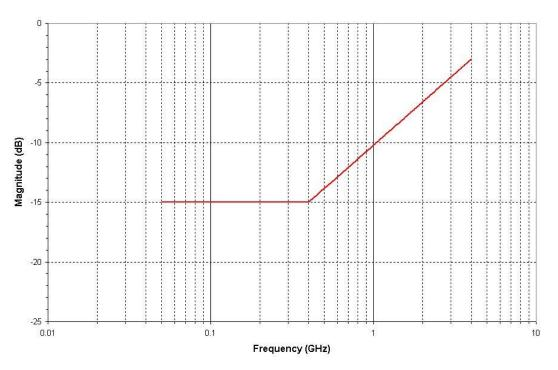
Figure 4-20: Mixed Mode Differential Return Loss (SDD11) of Reduced Bit Rate Cable
