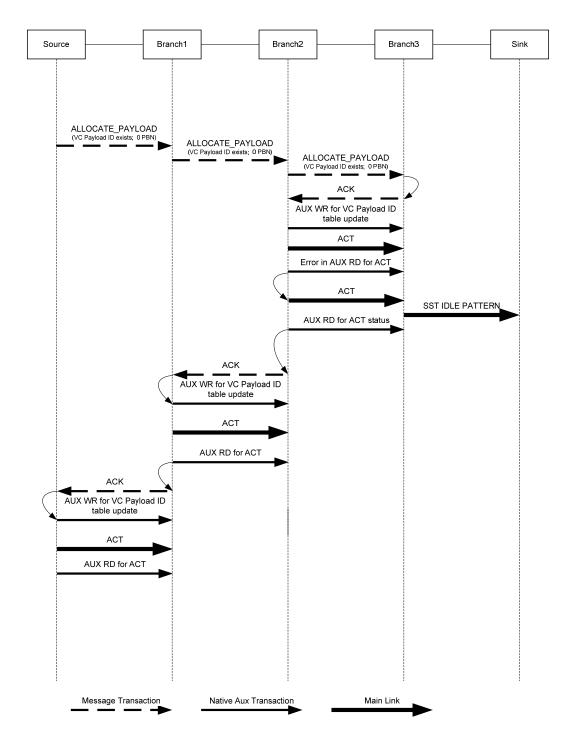
Figure 2-82: Timing Sequence for Deleting a Payload with an Error
