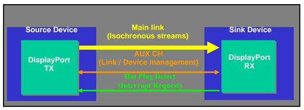
Figure 1-1: DisplayPort Data Transport Channels
