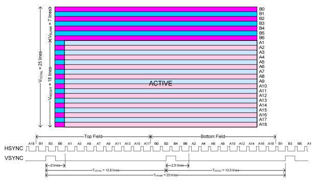
Figure 2-19: Interlaced Video Format/Timing for Odd Number of Lines per Frame
