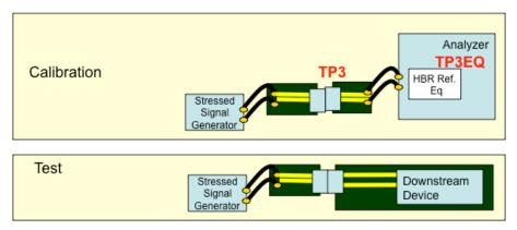
Figure 3-7: HBR Downstream Device Compliance Test Configuration
