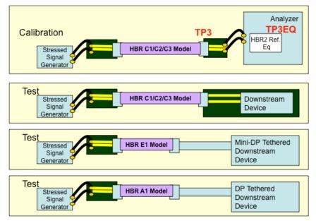
Figure 3-5: HBR2 Downstream Device Compliance Test Configuration
