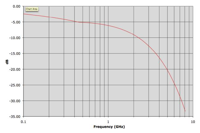
Figure 4-10: Mixed Mode Differential Insertion Loss for HBR Cable Assembly Type C1, C2 and C3
